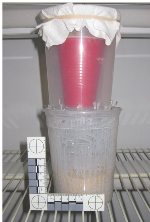
Fig. 1 Specialized rearing container designed to segregate feeding larvae from wandering larvae in order to nondestructively sample pupae [17]
